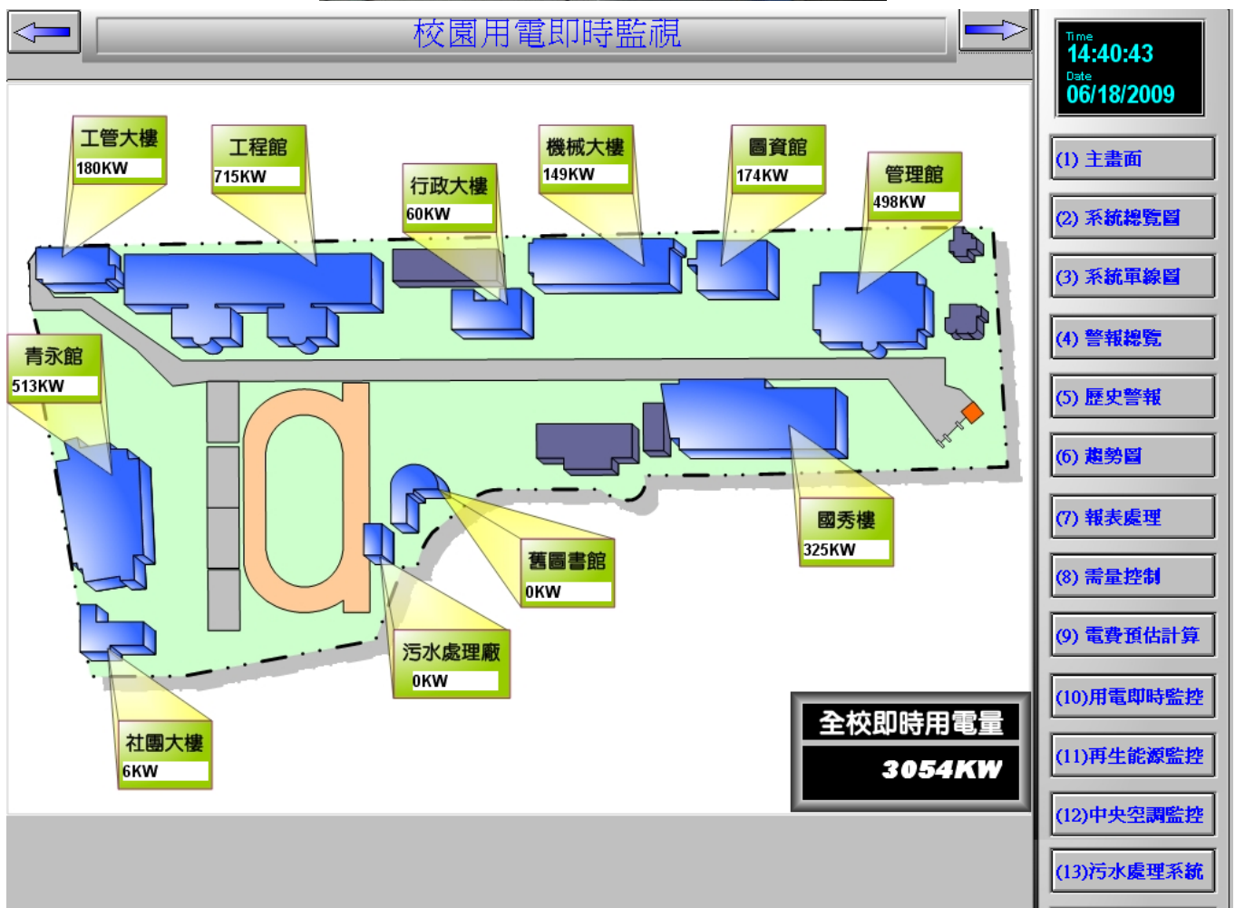
Campus electricity real-time monitoring system
